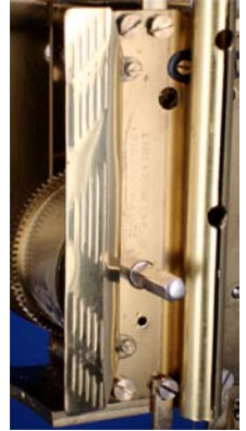
Edgar Henn's movement with side extensions fitted.
